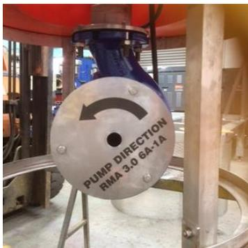
To change pump rotation, you will need to change the wiring within the electrical 3 phase connection to match the supply of the 3 phase power as well as the correct rotation on the pump.
