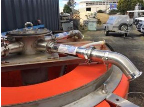
All models are fitted with a lifting hook in the middle of the top of the product. Note the hook in the centre top of the product in manufacture to the left.
