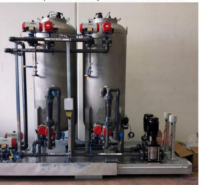
Optimised Velocity AFM Filters on first skid.
