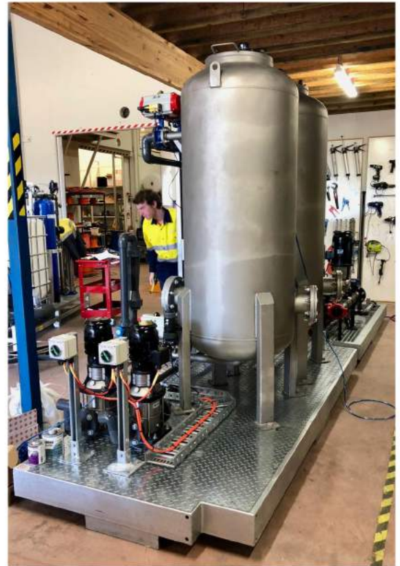
Combined skids during fabrication.
